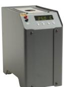
Fluke Calibration 9103 and 9140 Field Dry-Well Calibrators beat every other comparable dry-well in the industry in performance, size, weight, convenience, ease of calibration, software, and price. The heating and cooling rate of each of these dry-wells is adjustable from the front panel, and thermal switches can be checked for actuation testing. Multiple-hole inserts are available for a variety of probe sizes.
