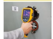
Combine with a Fluke ClirVu™ Infrared Window to conduct thermal inspections without having to open the electrical panel.
