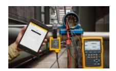
When you combine the Fluke 154 Communicator with a Fluke 750 Series Documenting Process Calibrator, or a Fluke 720 Series Multifunction Process Calibrator you have a complete HART calibration and configuration solution.
